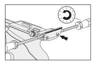
The depth of the rear sight leaf is variably adjustable from 1.8 to 2.6 mm.
